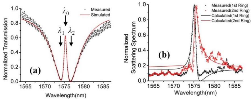
Fig. 3. Transmission and scattering spectra of the dual-ring resonator. (a) The measured (black dots) and fitted transmission spectra (the red line) [17].  $\lambda_0$  is the central wavelength of the supermode.  $\lambda_1$  and  $\lambda_2$  are the resonance wavelengths of the two individual rings. (b) The normalized scattering spectra for the two rings (red and black dots) and the spectra calculated using the parameters obtained from the fitting shown in (a) (red and black lines).
