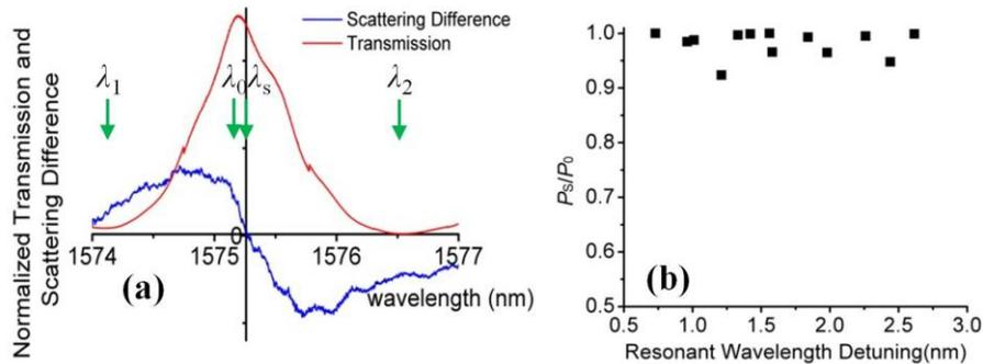
Fig. 4. (a) Measured transmission spectrum (the red line) and scattering difference (the blue line) near the central wavelength ( $\lambda_0$ ).  $\lambda_S$  is the wavelength where the scattering difference crosses zero (b) Power efficiency at different resonance wavelength detuning  $\lambda_2 - \lambda_1$ .  $P_S$  is the optical output power at  $\lambda_S$  and  $P_0$  is the optical output power at  $\lambda_0$ .
