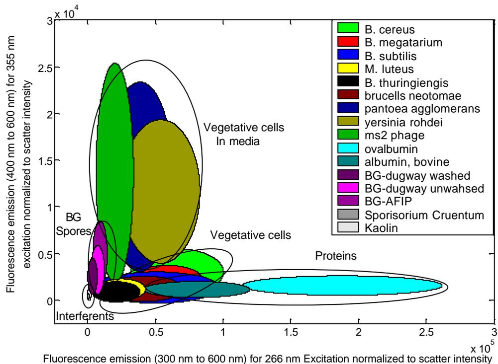
Fig. 4. Scatter plot distribution of the 355 nm-excited fluorescence versus the 266 nm-excited fluorescence for the 16 samples listed in Table 1. The ovals represent the probability that a particle of the indicated type will fall within that range.
