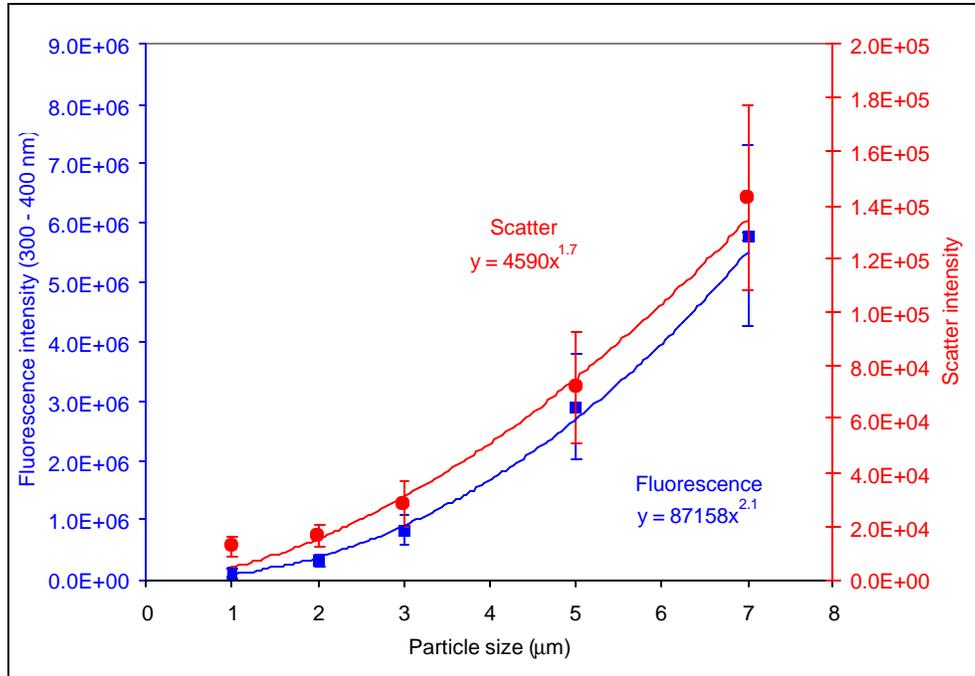
Fig. 2. Plots of the elastic scattered light and fluorescence intensity as a function of particle size for un-doped polystyrene spheres showing a cross-sectional area dependence on particle size.
