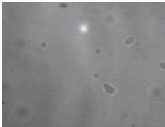
Fig. 5 (2.6MB) Movie (monochrome) of simultaneous two-photon excitation fluorescence and femtosecond optical tweezing of dye-doped 1.28  $\mu\text{m}$  polymer microspheres. While tweezing of the same microsphere is maintained, the fluorescent signal is turned off by simply switching the titanium-sapphire source laser from the femtosecond regime to the cw regime. This procedure is entirely reversible ([3.5MB version](#)).
