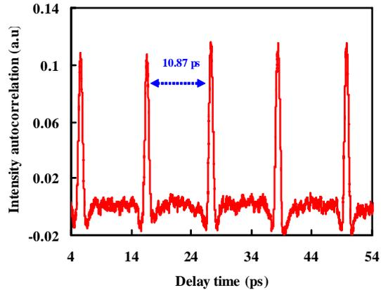
Fig. 3. Optical intensity autocorrelation pulse trains with the periodic time of 10.87 ps, which corresponds to a repetition rate of 92 GHz when the injection current is 60 mA.
