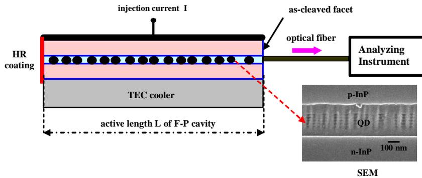
Fig. 1. Experimental set up of a passive single-section InAs/InP quantum dot mode-locked laser (MLL).
