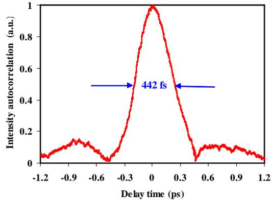
Fig. 4. Optical intensity autocorrelation trace with second-order autocorrelation measurements. Assuming a Gaussian pulse shape, the real pulse duration of the QD MML is estimated at 312 fs when the injection current is 45 mA at a temperature of 18°C.
