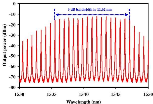
Fig.2. Optical spectrum of a passive single-section InAs/InP QD F-P mode-locked laser with an active length of 456  $\mu\text{m}$  and ridge width of 2.5  $\mu\text{m}$  at an injection current of 45 mA.
