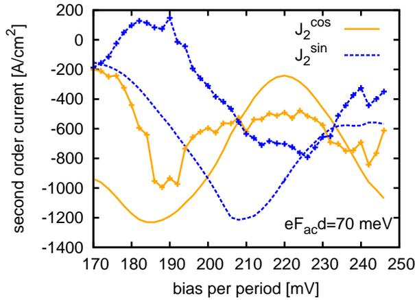
Fig. 6. Current response at  $2\omega$  in terms of the cosine and sine part respectively, from the NEGF model (solid lines). These are compared with the results from Eq. (5) using occupations and dipole matrix elements from our nonequilibrium states (connected dots). To compare directly to Eq. 4, the negative particle current, appropriate for electrons, is shown. The ac field strength is held constant at  $eF_{ac}d = 70$  meV.
