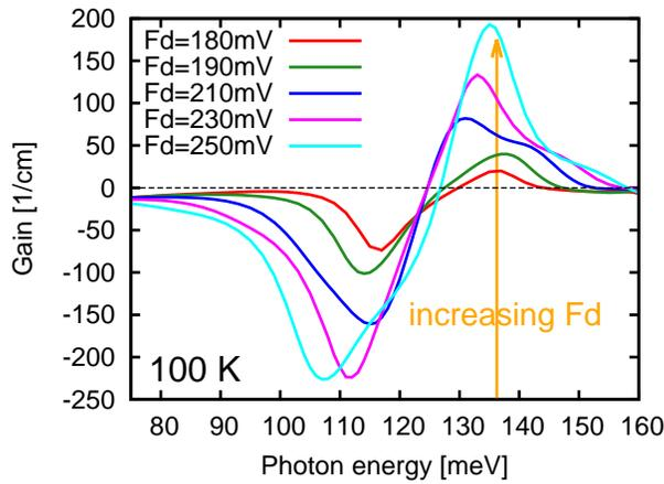
Fig. 3. Gain at weak ac field simulated at the bias points marked in Fig. 2. The orange arrow indicates the photon energy 136.25 meV corresponding to the fundamental wavelength of  $9.5 \mu\text{m}$ , as well as increasing bias.
