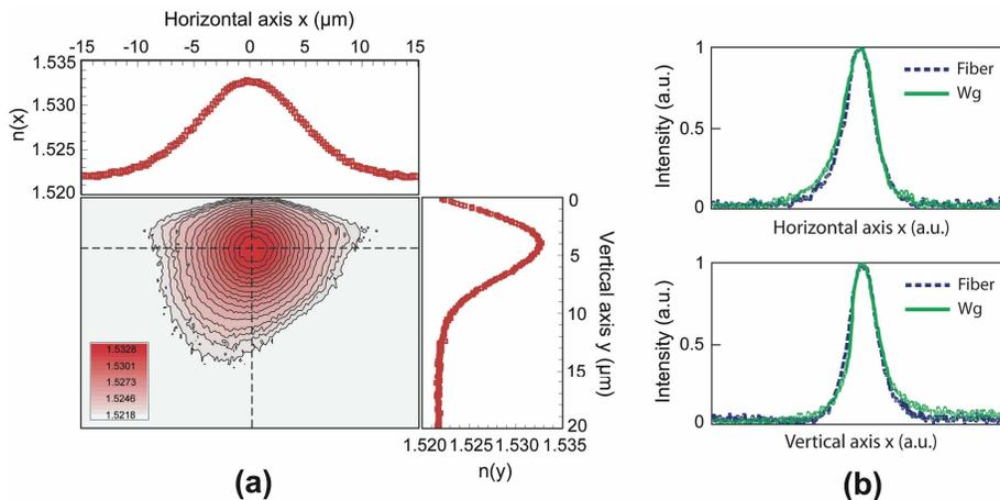
Fig. 1. (a). Typical waveguide refractive index profiles. (b) Typical near-field mode profiles of the waveguide compared to near-field mode profiles of standard SMF-28 fiber at 1550 nm.
