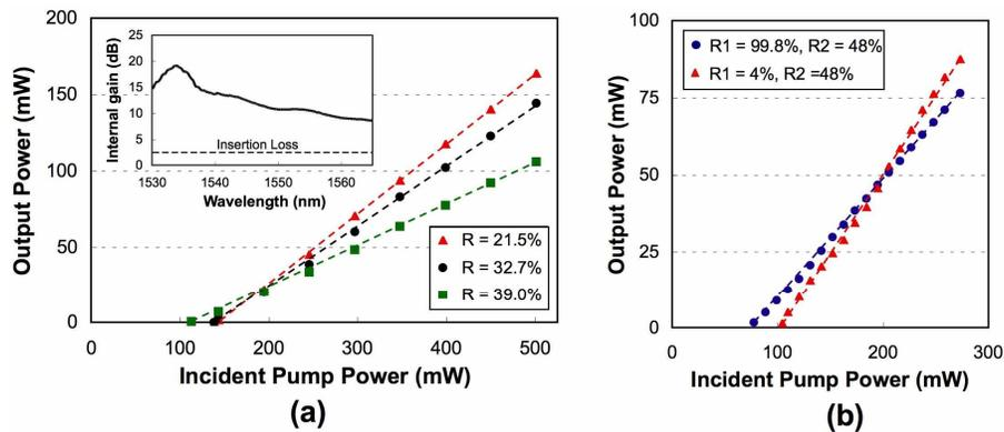
Fig. 6. (a). Laser output power (in multimode operation) vs. pump power (double-end pumping) for the 45-mm long active waveguide for three different output couplers. Inset shows the small-signal internal gain and insertion losses of the 45-mm long active waveguide under 500 mW total incident pump power (double-end pumping scheme). (b) Laser characteristics of the 60 mm long laser cavity based on a 50-mm long active waveguide specially designed to allow efficient single-end pumping at 980 nm.
