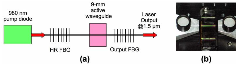
Fig. 2. (a). Schematic of waveguide laser set-up. (b) Picture of the 9-mm waveguide laser.
