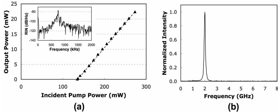
Fig. 4. (a). Single mode laser output power as a function of pump power. Inset shows RIN spectrum at 22 mW output power. (b). Fabry-Perot spectrum of the single mode laser. The frequency offset shows drift without mode-hopping.
