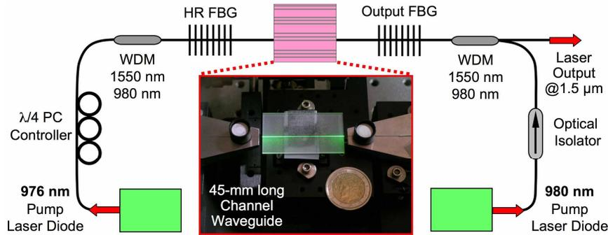
Fig. 5. Laser cavity setup for high power waveguide laser experiments. PC: polarization controller. Picture shows a 45 mm long active waveguide butt-coupled to FBG fibers under double-end pumping.
