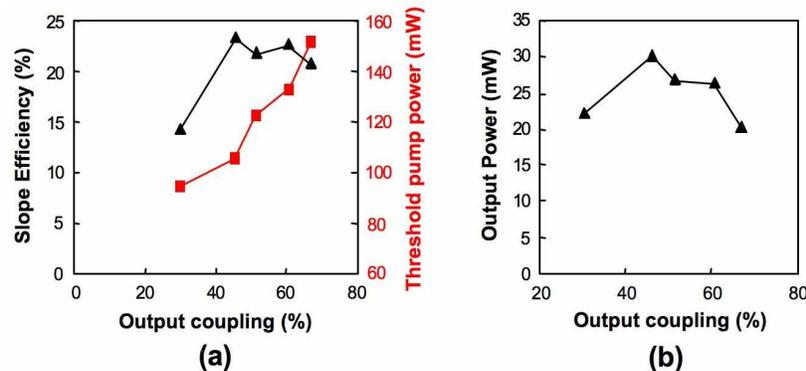
Fig. 3. (a). Slope efficiency (triangles) and pump power threshold (squares) vs. output coupling. (b) Maximum output power vs. output coupling.
