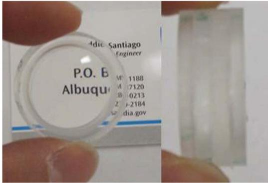
Fig. 1. (Left) ADPL focusing on a business card. (Right) Side view of the ADPL showing support rings.
