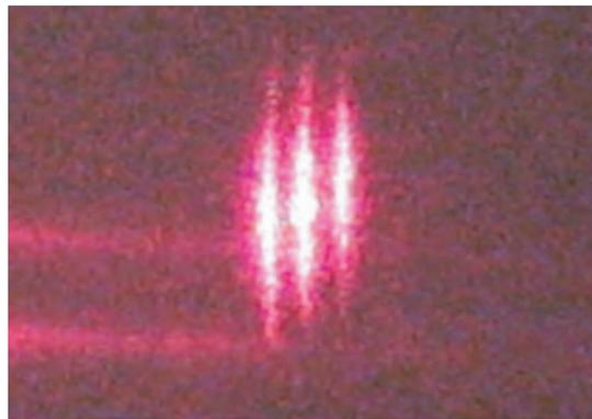
Fig. 7. Double phase conjugated image observed on the screen of three independent emitters of a laser diode bar.
