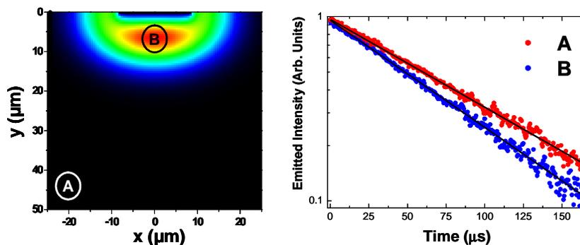
Fig. 2.- Fluorescence decay curve of the  $^4F_{3/2}$  metastable state of Nd<sup>3+</sup> ions in the LiNbO<sub>3</sub> bulk and RPE channel waveguide (red and blue points, respectively). Solid lines correspond to a single exponential fit. The spatial location at which each curve was measured is indicated in the graph on the left.
