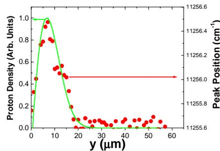
Fig. 5.- Energy position of the main luminescence peak within the  ${}^4F_{3/2} \rightarrow {}^4I_{9/2}$  fluorescence band as a function of the y position (red points). Green line is the proton density as obtained from the 2D calculations included in Fig. 1(b).
