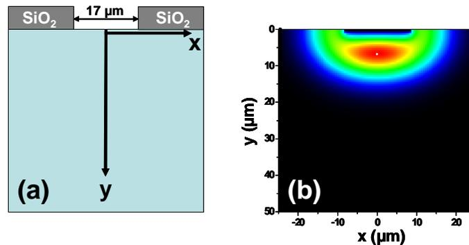
Fig. 1. (a).- Nd:LiNbO<sub>3</sub> sample with silica mask channel opening. Reference axis used in this work are indicated. (b).- Two dimensional calculation of the proton density in the waveguide as obtained by using the imaginary distance beam propagation method
