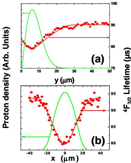
Fig. 3.-  ${}^4\text{F}_{3/2}$  lifetime as a function of both  $y$  and  $x$  positions ((a) and (b), respectively). Green line corresponds to the proton density along the  $y$  and  $x$  scan directions.
