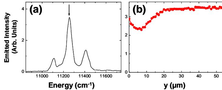
Fig. 4. (a).-  ${}^4F_{3/2} \rightarrow {}^4I_{9/2}$  micro fluorescence spectrum obtained under continuous wave excitation. (b).-  ${}^4F_{3/2} \rightarrow {}^4I_{9/2}$  emitted intensity as a function of the y position.
