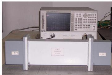
Fig. 2. Experimental setup for the scattering parameters measurement in rectangular waveguide
