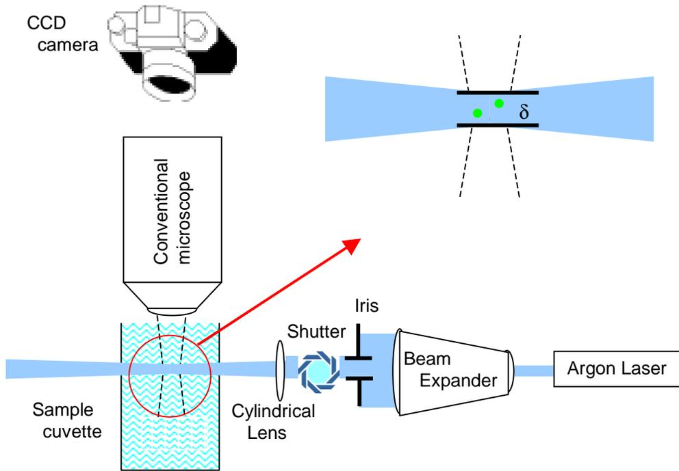
Figure 1: Thin light sheet microscopy (TLSM), schematic diagram.
