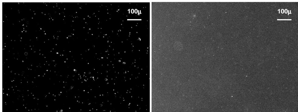
Figure 3 (a): Sample illuminated with the thin light sheet illumination. (b) Same sample with a broad beam illumination. Marine bacterial isolates in  $0.22 \mu\text{m}$  filtered seawater, stained. Particle size cannot be scaled due to sensor blooming. Particles appear about 1.7 times larger than their actual size.
