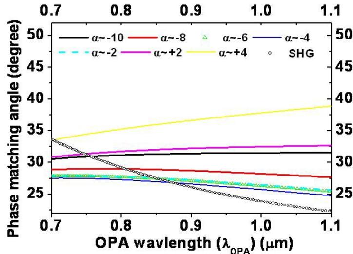
Fig. 3. Theoretical calculation on the relationship of phase-matching angle of SFG and SHG as a function of wavelength of OPA indicating the coexistence of SFG and SHG near the degenerate point of OPA at 810 nm.
