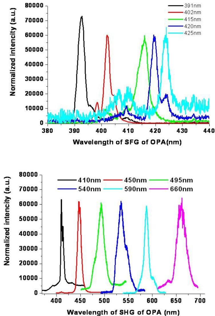
Fig. 2 Spectra of cascaded SFG (up-figure) and SHG (bottom-figure) of NOPA at various BBO orientations. The spectra were taken at a seeding angle of 8 degree.
