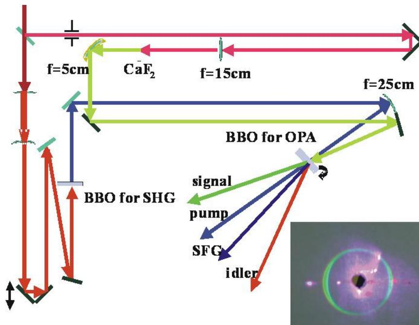
Fig. 1 Experimental setup of the OPA-SHG/SFG. The bright spot on the left of the parametric superfluorescence ring is the SHG component and the central spot is a pinhole to let the residual pump beam go through to avoid saturating the CCD camera. The spot between the pump of OPA and the SHG is the SFG component. The image is taken with a seeding angle of 8-degree.
