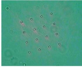
Fig. 2. (0.6 MB) Movie of  $4 \times 4$  array of traps on  $5 \mu\text{m}$  pitch with 700 mW total input power showing capture of final trap.
