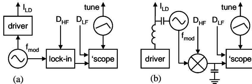
Fig. 2. Instrumental configuration used for (a) WMS and (b) FMS detection.  $I_{LD}$ : Injection current to DBR laser, tune: ramp signal to DBR tuning controller,  $D_{HF}$ : fast mid-IR detector signal,  $D_{LF}$ : slow mid-IR detector signal, driver: DBR laser injection current supply, 'scope: digital storage oscilloscope.
