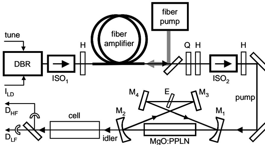
Fig. 1. Optical configuration for WMS and FMS experiments. DBR: multi-section DBR diode laser,  $ISO_1$ : 60dB isolator,  $ISO_2$ : 30dB isolator, Q and H: quarter- and half-wave plates,  $M_{1-4}$ : OPO cavity mirrors, E: intracavity etalon, tune: tuning input to DBR laser,  $I_{LD}$ : DBR laser injection current supply,  $D_{HF}$ : fast mid-IR detector output,  $D_{LF}$ : slow mid-IR detector output. Electrical connections relate to instrumental configuration shown in Fig. 2.
