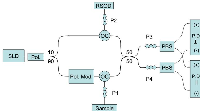
Fig. 1. Schematic of the PS-OCT system. Abbreviations: SLD, super luminescent diode; Pol., linear polarizer; Pol. Mod., polarization modulator; 90/10, 50/50, fiber couplers; RSOD, rapid scanning optical delay; OC, optical circulator; P#, polarization paddles; PBS, polarization beam splitter; P.D., photodetector.
