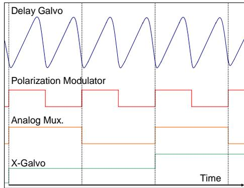
Fig. 2. Synchronized signals used to control the RSOD delay galvanometer (blue), the polarization modulator (red), the analog two-channel multiplexer (orange), and the x-galvanometer (green). Fringe data was collected during the rising slope of the pseudo-sawtooth delay waveform (blue).
