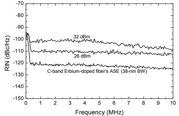
FIG. 3. Measured relative-intensity noise levels of the EDF's ASE-seeded CW SC for various power levels of the amplified 3-nm-bandwidth ASE beam together with that of C-band EDF's ASE.
