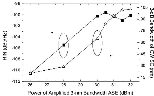
FIG. 4. RIN level and spectral bandwidth of the EDF's ASE-seeded CW SC as a function of the amplified 3-nm-bandwidth ASE beam power.
