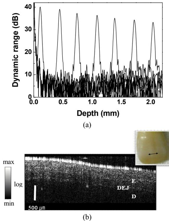
FIG. 5. (a) Measured axial point spread functions at various optical-length differences. (b) OCT image of a human tooth sample. The brighter regions correspond to the areas with a larger backscattered intensity (unit: dB). A picture of the sample surface is shown in the inset. The double-headed arrow indicates the sample's scan range for the OCT image. Abbreviations: E, enamel; D, dentin; DEJ, dentoepithelial junction.
